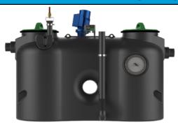
Model MIX is equipped with Grease alarm is indicating when the maximum accumulated grease is reached. Before emptying, Mixer actuated for blending grease, water and solid layers thus facilitating emptying of the separator. A special Extraction pipe is provided for the emptying of grease separator by the vacuum truck. After complete disposal, the separator is filled-up with freshwater.
