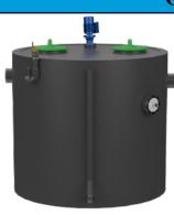
Model MIX is equipped with Grease alarm is indicating when the maximum level of accumulated grease is reached. Before emptying, Mixer actuated for blending grease, water and solid layers thus facilitating emptying of the separator. A special Extraction pipe is provided for the emptying of grease separator by the vacuum truck. After complete disposal, the separator is filled-up with freshwater.
