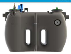
Model MIX is equipped with Grease alarm is maximum indicating when the accumulated grease is reached. Before emptying, Mixer actuated for blending grease, water and solid layers thus facilitating emptying of the separator. A special Extraction pipe is provided for the emptying of grease separator by the vacuum truck. After complete disposal, the separator is filled-up with freshwater.
